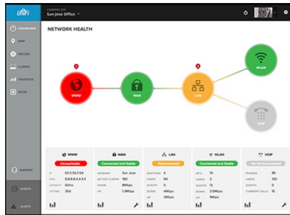
Figure 5.2: UniFi controller dashboard [18]
